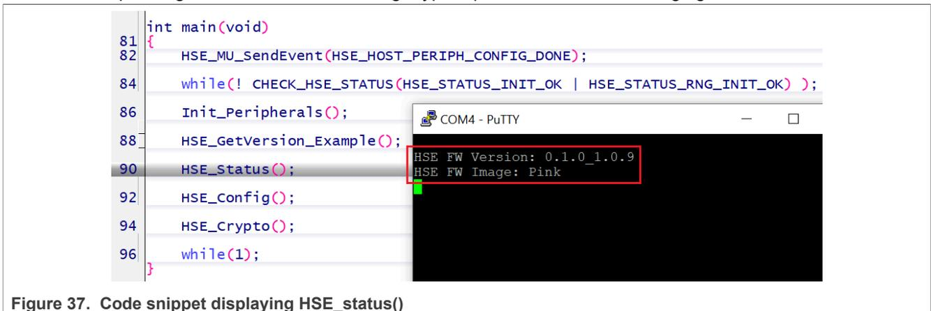
Figure 37. Code snippet displaying HSE\_status()
