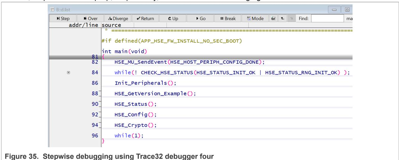
Figure 35. Stepwise debugging using Trace32 debugger four
