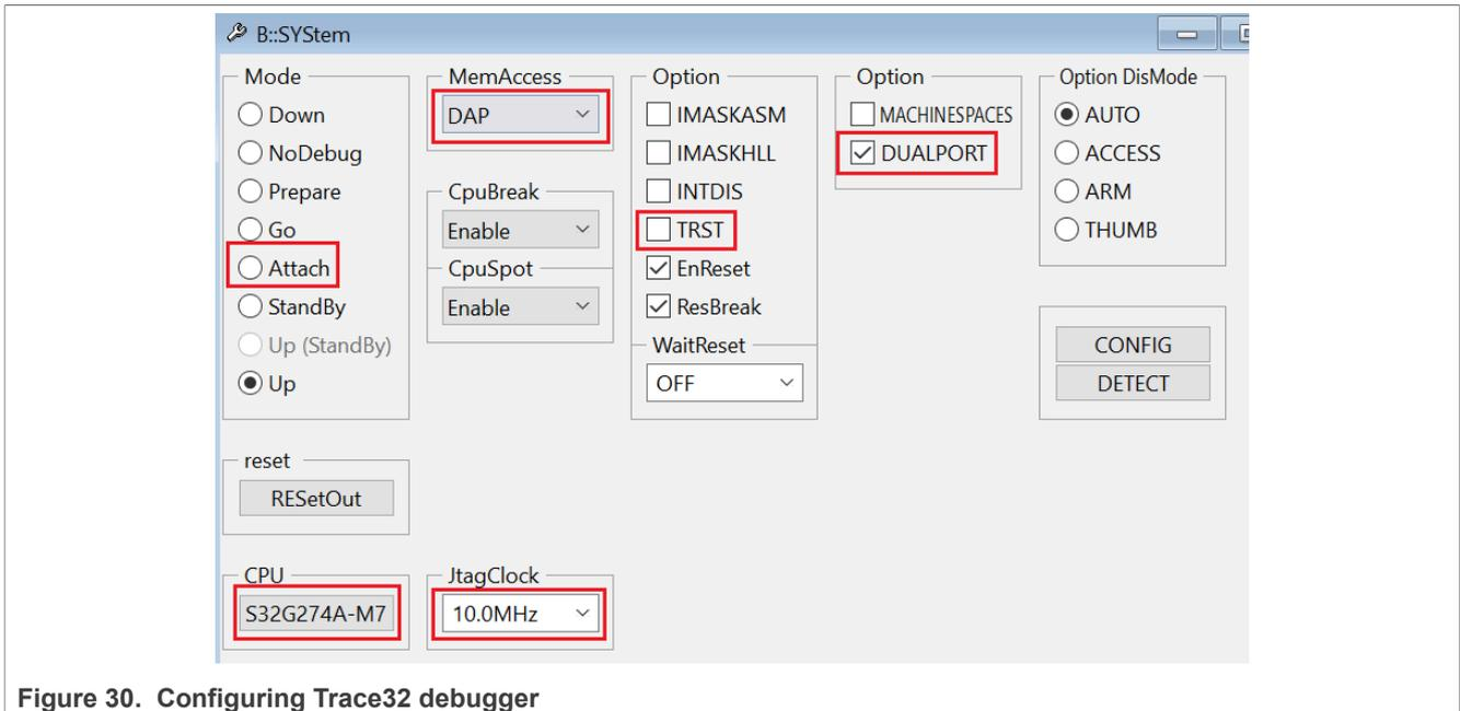
Figure 30. Configuring Trace32 debugger
